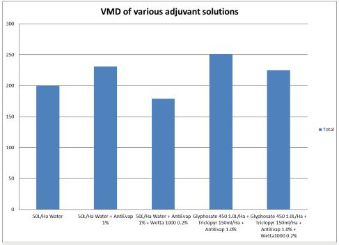
**Chart 1:** Oil based adjuvants such as ANTIEVAP® have a positive effect on increasing droplet size versus non-ionic surfactants. (Source: USDA 2014)
