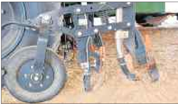
□ The seeding kit system set-up for delivery of the SE14 moisture and retention agent near the seed.
